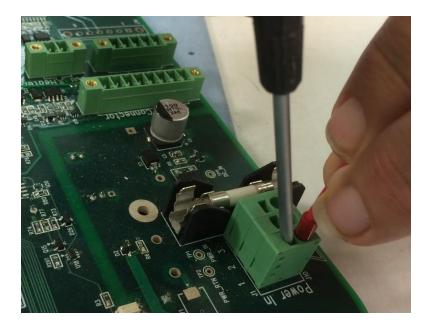
**Note:** It is important to confirm that the power wiring is secure in order to prevent erratic operation of the equipment.
