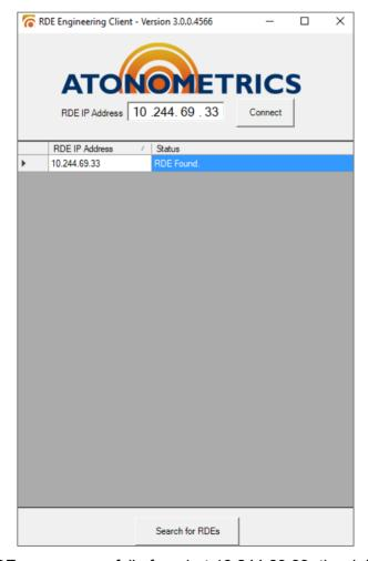
As shown here, an RDE was successfully found at 10.244.69.33, the default IP address for the RDE. Once the RDE is found, press "Connect."
