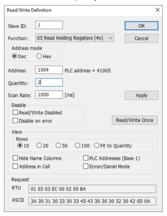
**Note:** Ensure that the box marked "PLC Addresses (Base 1)" is unchecked. If this box is checked, you must add 1 to the register addresses listed in the RDE300 User Guide.
